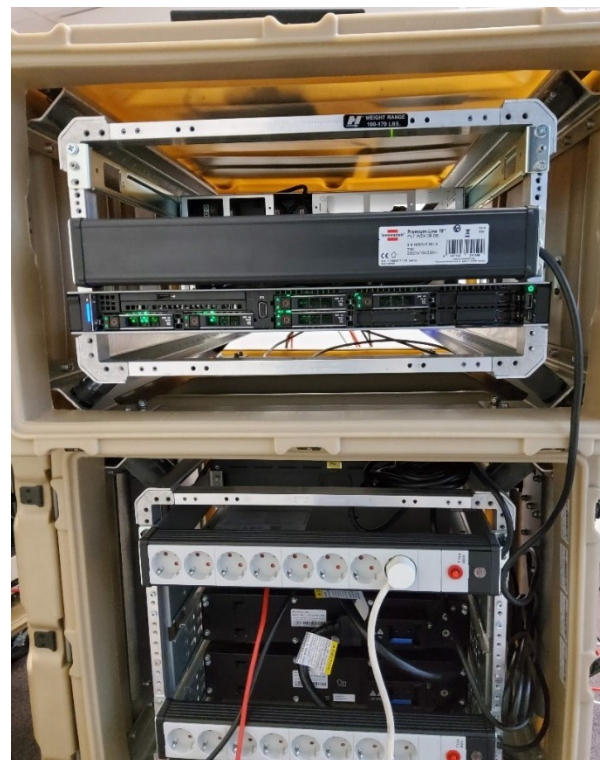
Figure 2-32 Back view of the Ruggedized, mobile edge data center with power-supply
