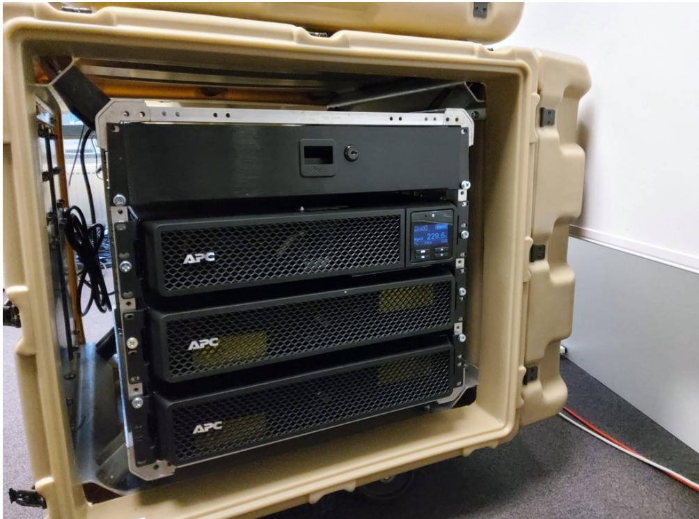
Figure 2-33 Front-view of the power supply in the Ruggedized, mobile edge data center
