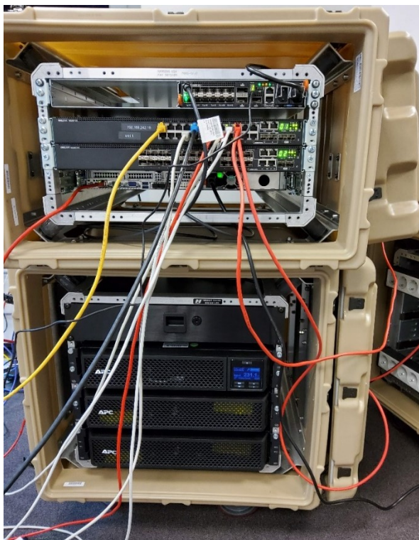
Figure 2-31 Front view of the compute storage and switching with UPS
