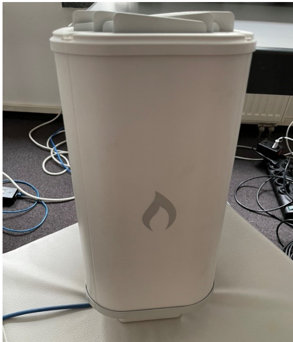
Figure 2-13 Ignite 60 GHz AP at FOKUS R&amp;D lab
