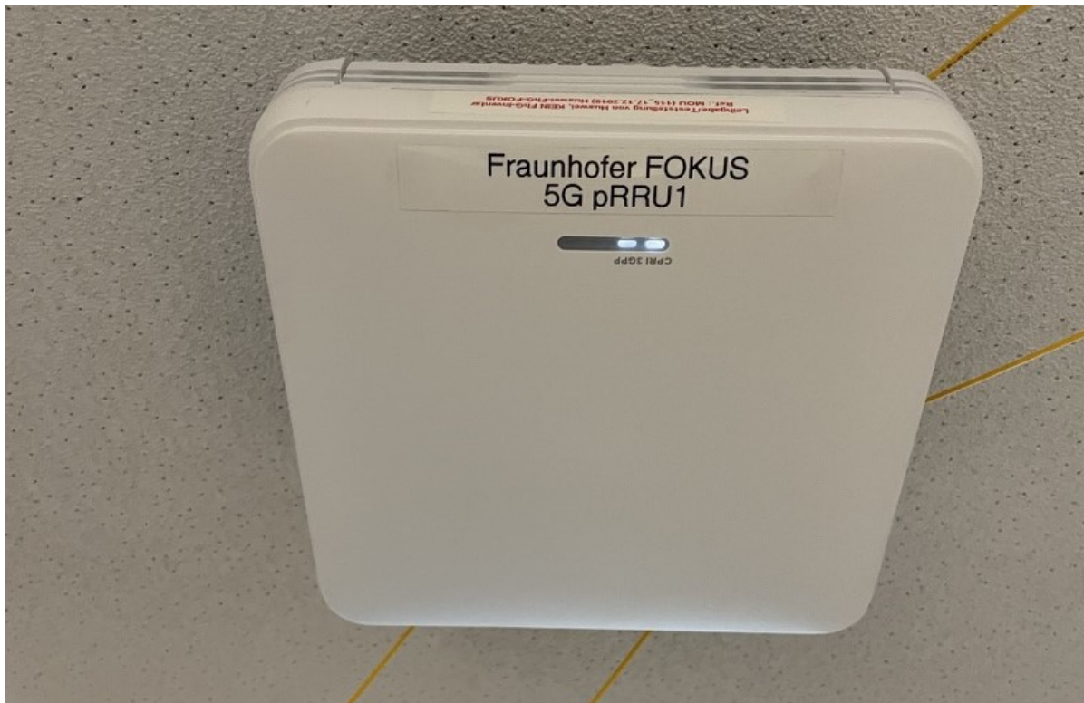
Figure 2-11 Huawei Remote Radio Head at FOKUS R&D lab
