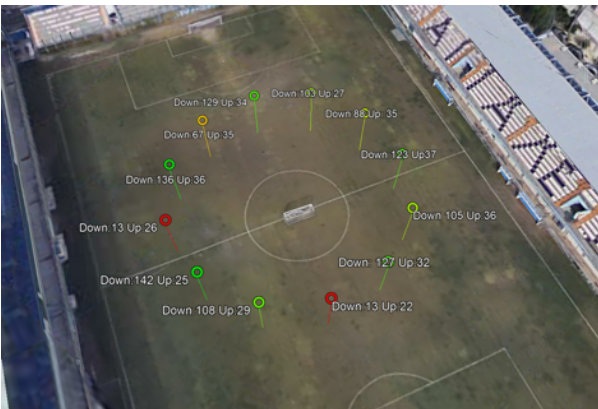
Fig. 4 Coverage area with uplink and downlink values
