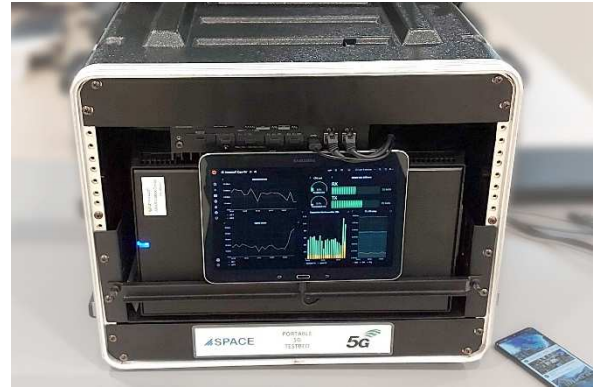
Fig.1. Portable “5G Hotspot” deployed at the satellite edge
