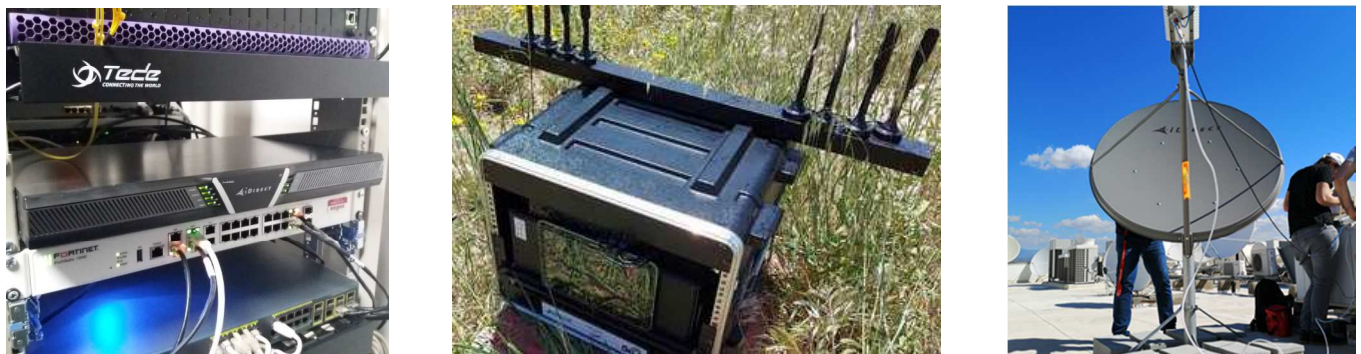
Fig. 1. Core data center (left), portable “5G Hotspot” deployed at the satellite edge (center), satellite link (right)
