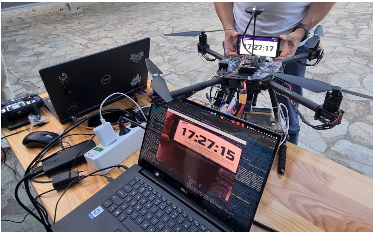
Figure 35 Video feed of the UAV Camera received from video clients showing the minimal latency
