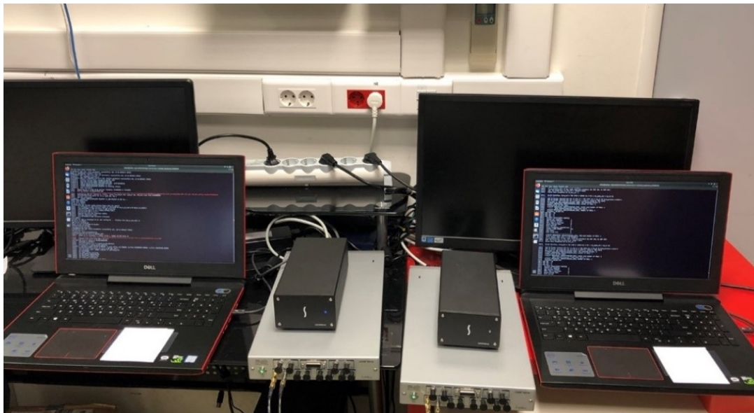
Figure 15 OAI gNB and OAI nr-UE utilized in noS1 mode (without core network)
