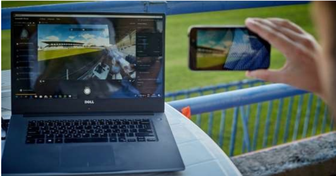
Figure 33 eMBMS reception of the 360° Camera feed
