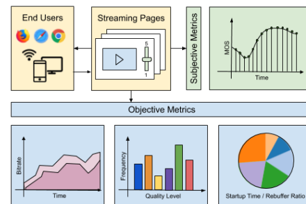
Figure 1: Approach for QoE-based analysis
