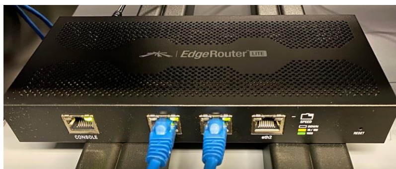
Figure 19. Colocation router installed for 5GENESIS at Makarios Earth Station
