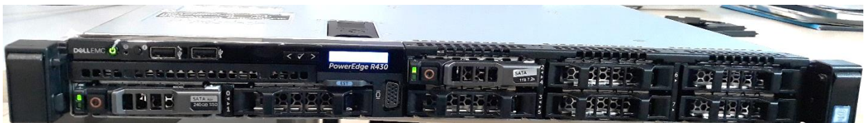
Figure 12. Dell R430 server, as building block of the Core Cloud Domain
