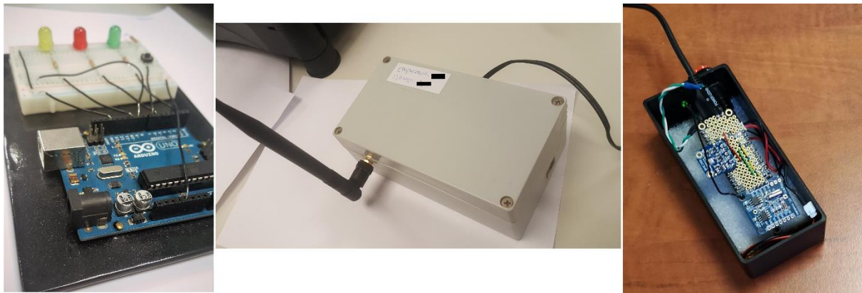
Figure 31: Arduino device with Colour LEDs, Physical Gateway LoRa compatible and LoRa device with sensors for UC2.
