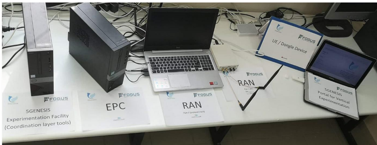
Figure 9 The end-to-end 4G set up
