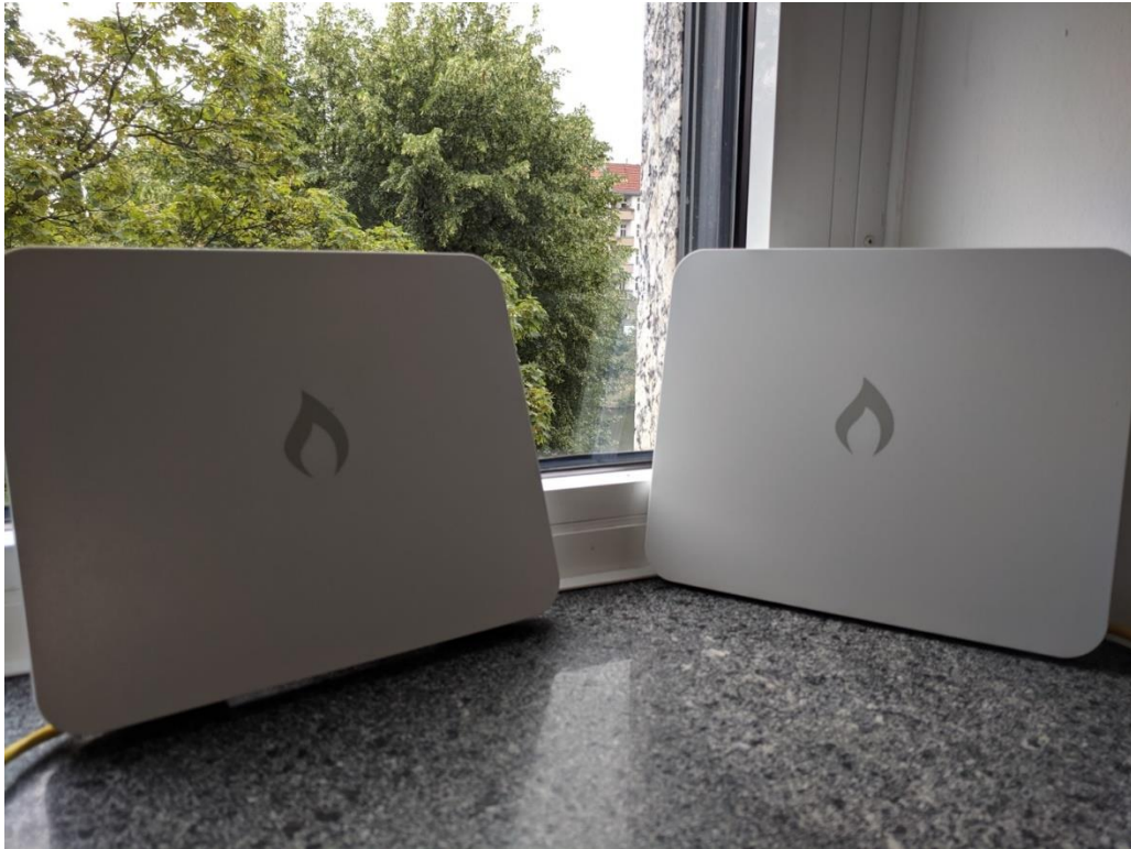
Figure 9-4 60 GHz MetroLinq mmWave system deployed at FOKUS for Phase 1
