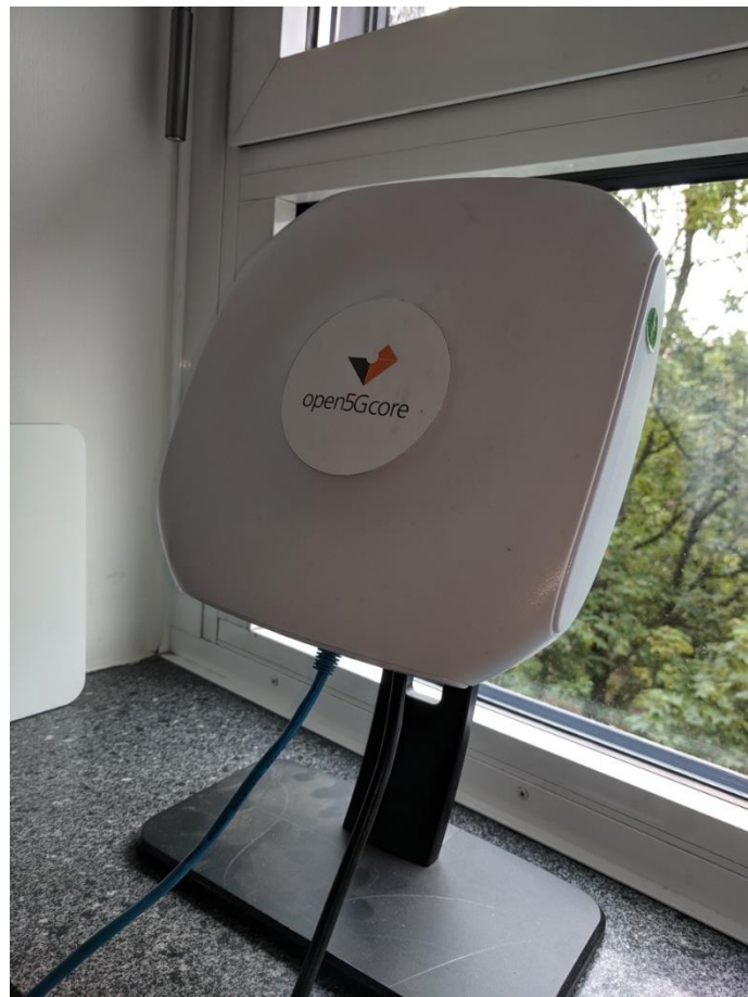
Figure 9-5 AirSpan LTE Femto Cell deployed at FOKUS for Phase 1
