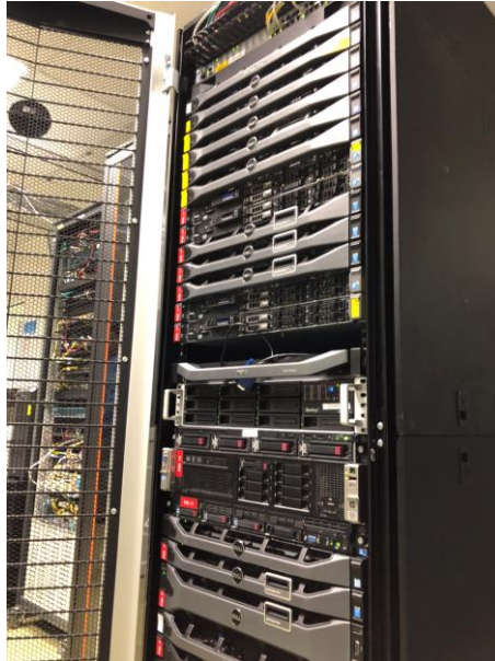
Figure 6-1 Athens platform compute nodes and ATH EPC deployed for phase 1
