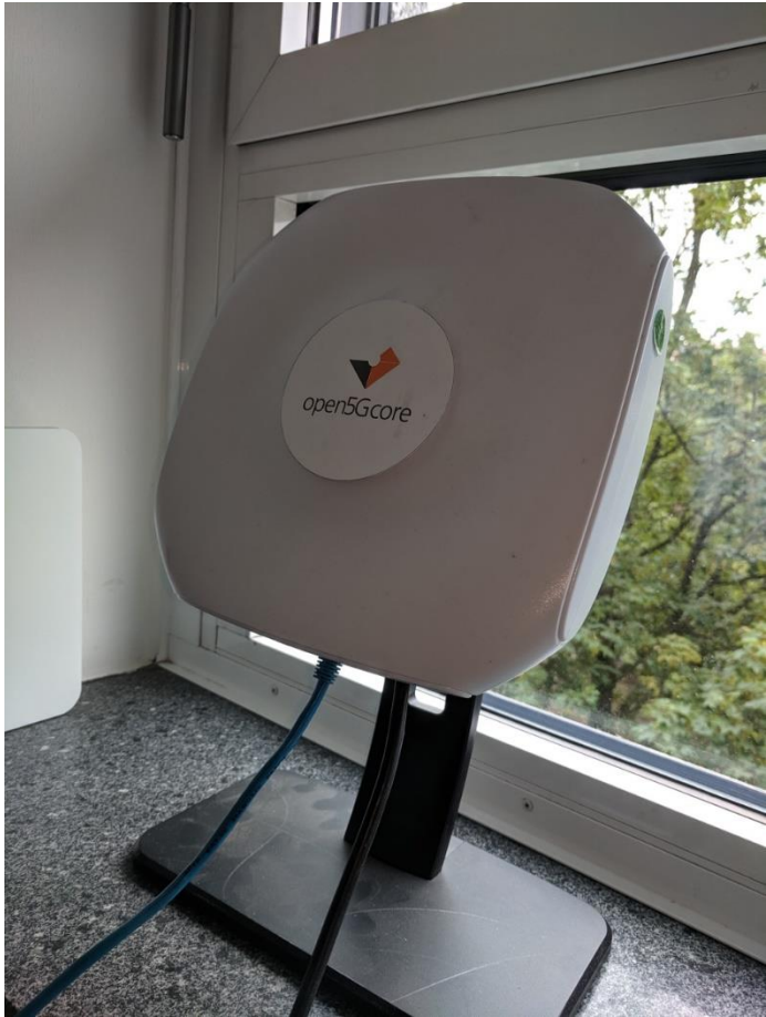
Figure 31 AirSpan LTE Femto Cell deployed at FOKUS for Phase 1
